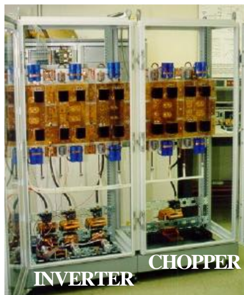
Figure 2.29. Experimental SMES PCS system.
